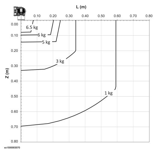
Extra load of 10 kg at the upper arm housing included in the load diagram.
