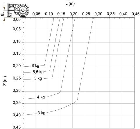
Extra load of 15 kg at the upper arm housing included in the load diagram.
