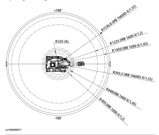
(A) Minimum turning radius axis 1 (all models)
