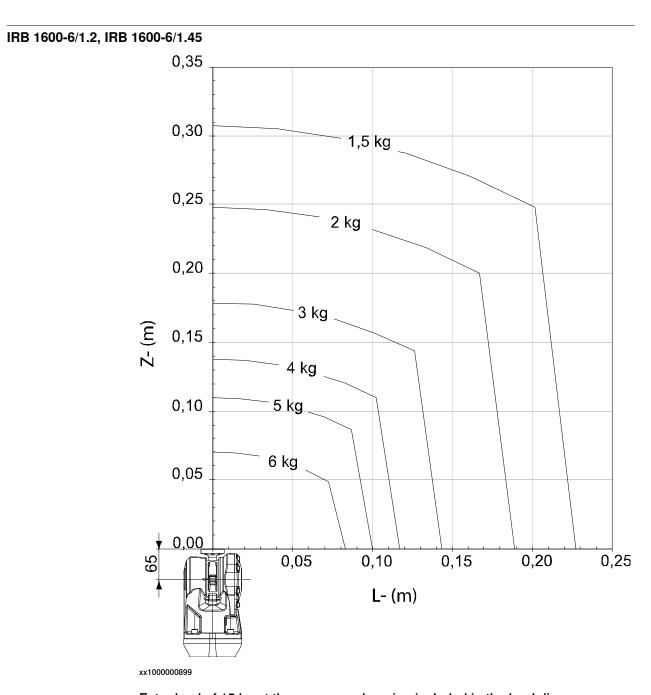
Extra load of 15 kg at the upper arm housing included in the load diagram.
