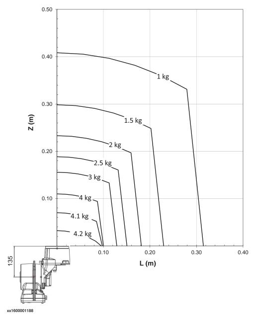
Extra load of 12 kg at the upper arm housing included in the load diagram.
