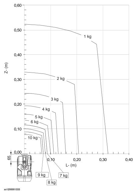
Extra load of 5 kg at the upper arm housing included in the load diagram.
